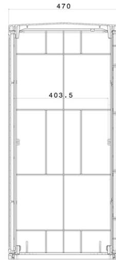
Based on the standard system of cabinet heights 1000 and 1300 mm (without stand) in the widths 805, 1135 and 1465 mm (with depth 320mm) GSAB delivers from now also all variants of the cabinets with width 805 and 1135 mm with a depth of **470 mm!**
