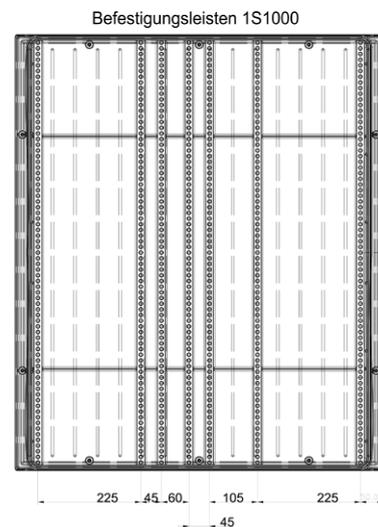
The innovative attachment system with rails on the rear of the cabinet was also applied for cabinet with depth 470 mm.
