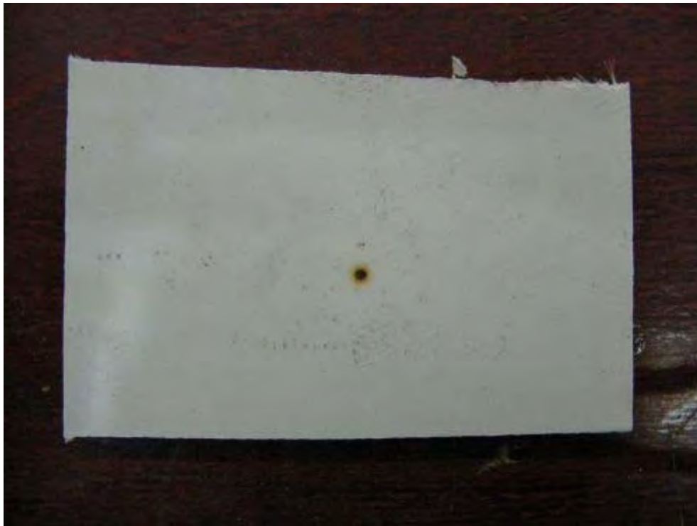
Photograph 11: Condition of test object after test after the glow-wire test
