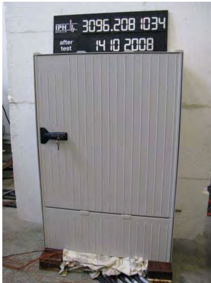
Photograph 2: Test object during temperature-rise test (front view)
