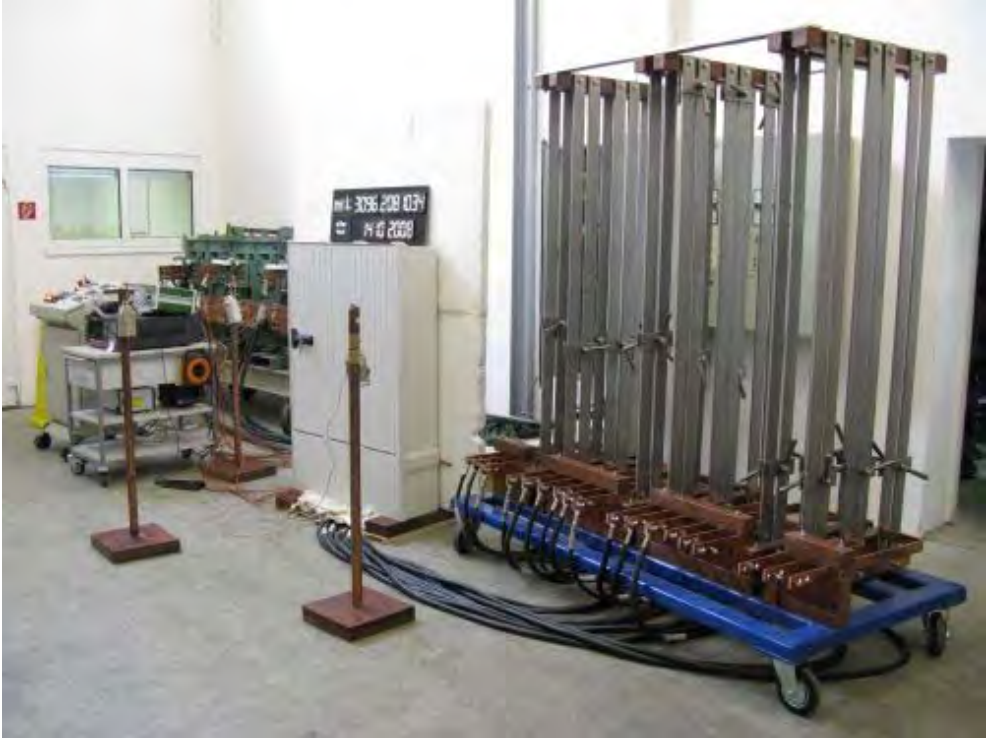
Photograph 1: Arrangement for the temperature-rise test
