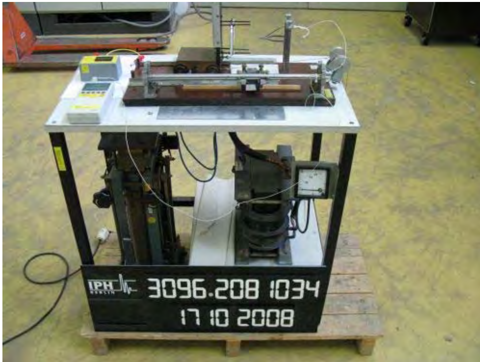
Photograph 9: Arrangement for glow-wire test
