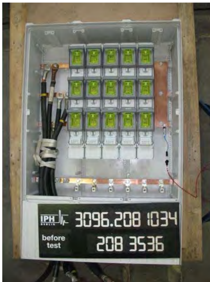
Photo 3: Arrangement for the short-circuit test of the main busbars (Condition of test object before short-circuit test)
