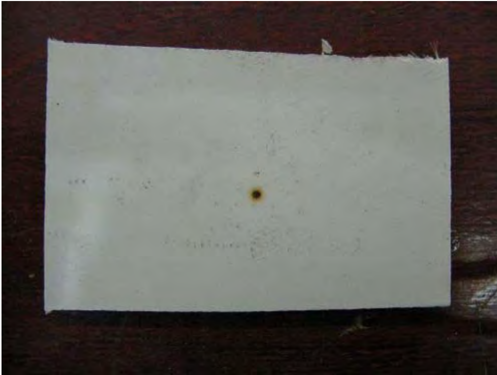
Photo 11: Condition of test object after test after the glow-wire test
