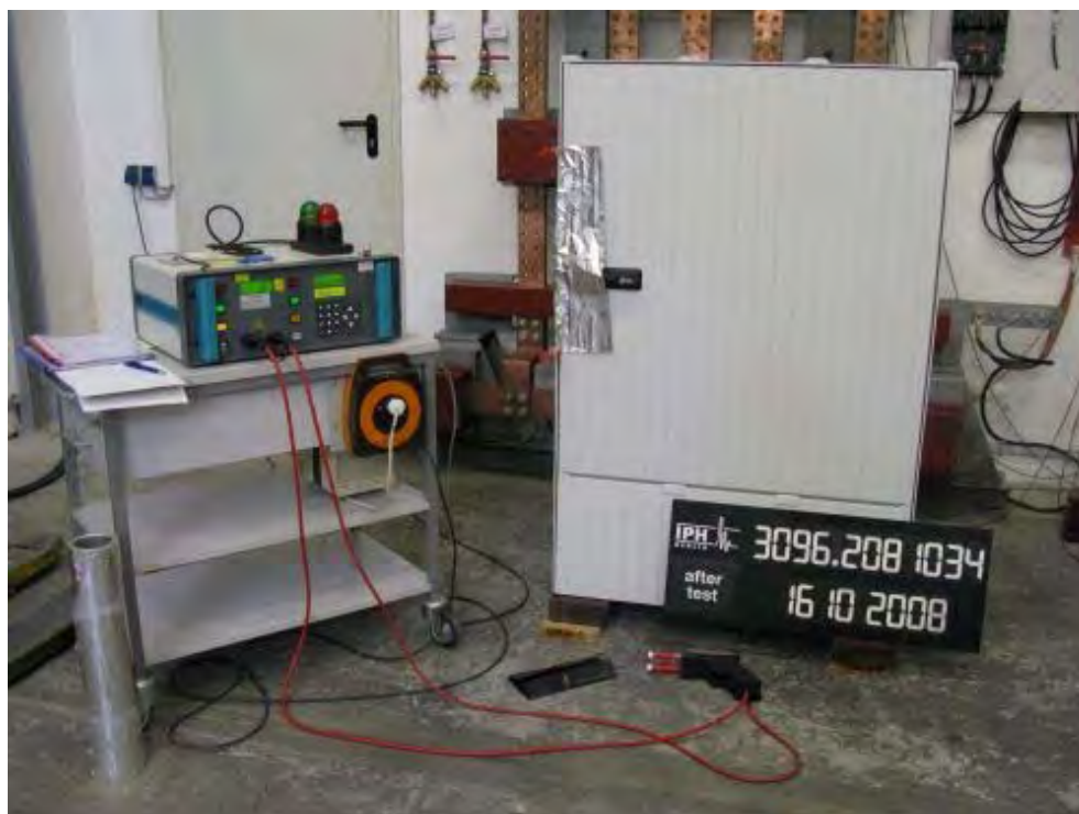
Photo 8: Arrangement for voltage test
