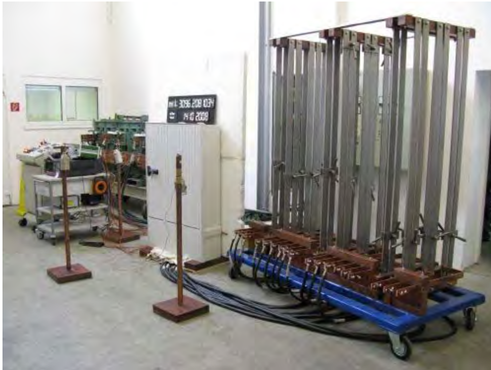
Photo 1: Arrangement for the temperature-rise test
