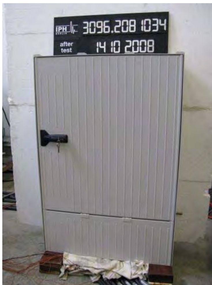
Photo 2: Test object during temperature-rise test (front view)
