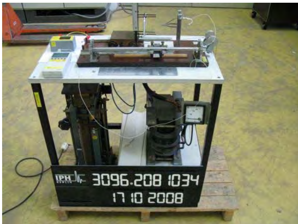
Photo 9: Arrangement for glow-wire test
